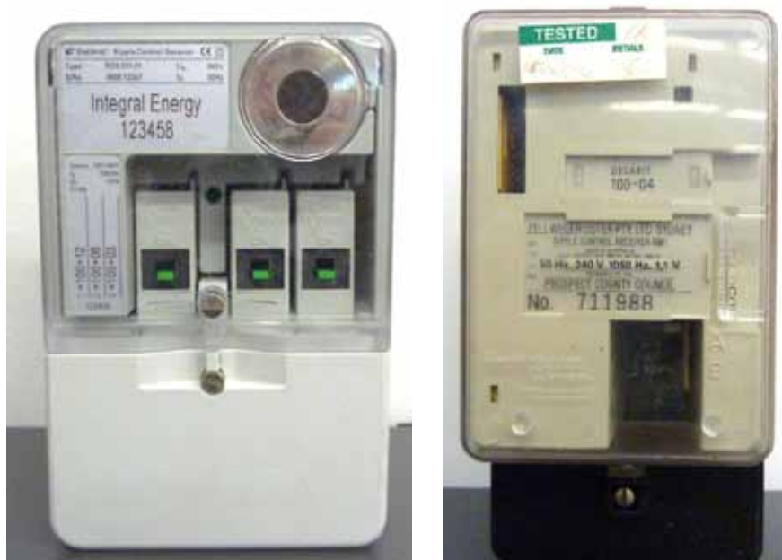
Figure 3.7: Photographs of Decabit Receiving Relays
