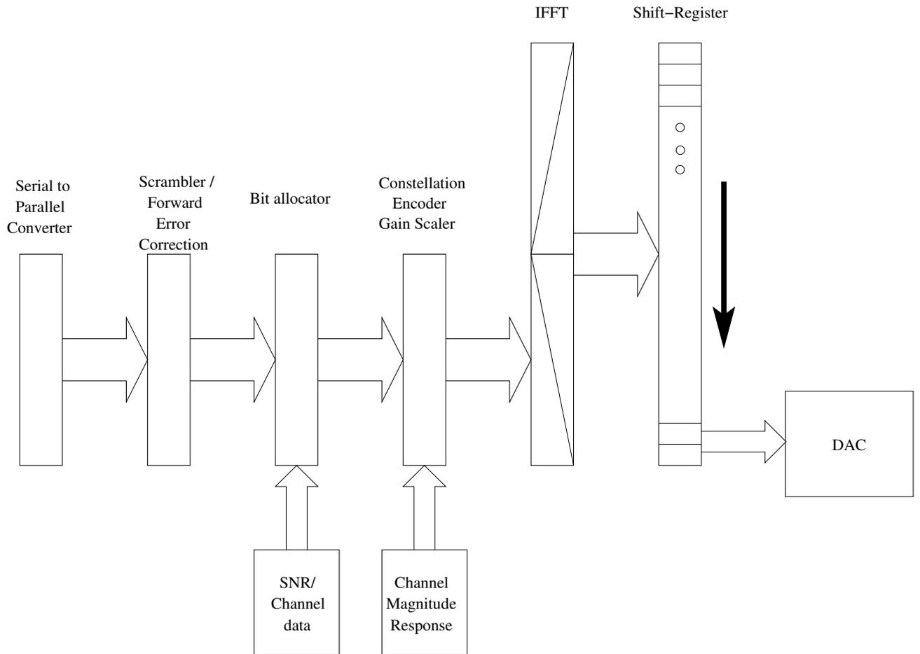
Figure 1: DMT Modulator - Block Diagram
