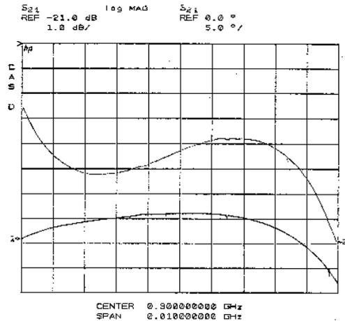
Fig.4.2 Magnitude and phase of the transfer function between RFin and RFout for frequency span of 10 MHz
