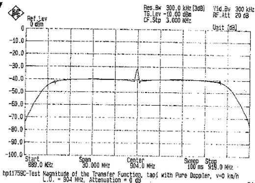
Fig.4.1 Magnitude of the transfer function between RF input and RF output for a frequency span of 30 MHz
