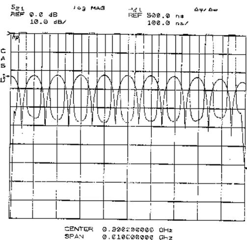
Fig.4.6 Magnitude and group delay of the transfer function between RF input and RF output A for a two-tap model with magnitudes differing by 1 dB and delays differing by 1 us
