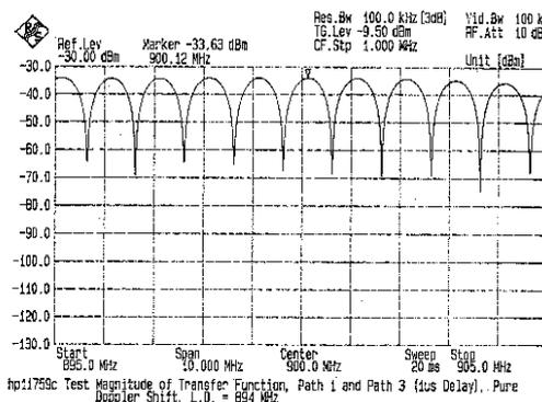
Fig.4.4 Magnitude of the transfer function between RF input and RF output for a two-tap model with equal magnitudes and delays differing by 1 us
