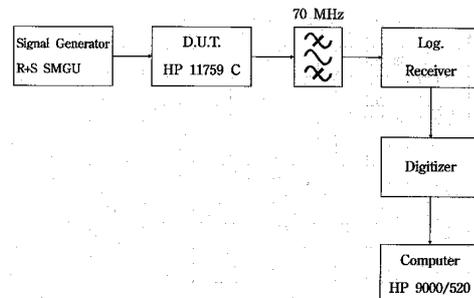
Fig.5.1 Set up for amplitude statistics measurements
