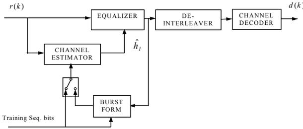
Fig 2. Iterative channel estimation feedback from equalizer [1]
