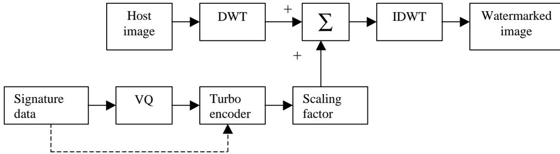
**Figure 1.** Block diagram of the encoder.
