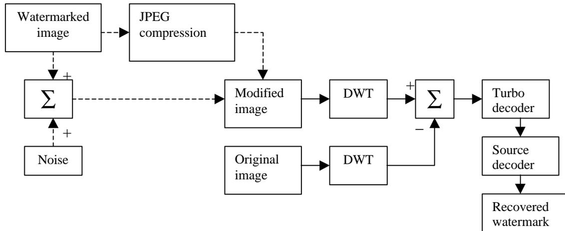
**Figure 2** Block diagram of the decoder
