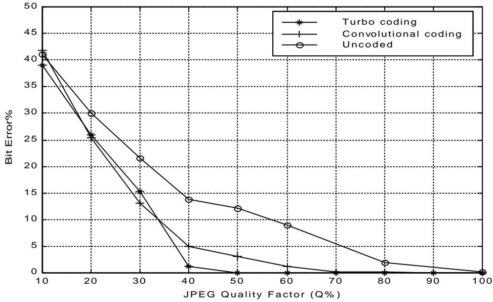
**Figure 5** Bit error rate versus JPEG compression for turbo codes, convolutional code, and uncoded messages.
