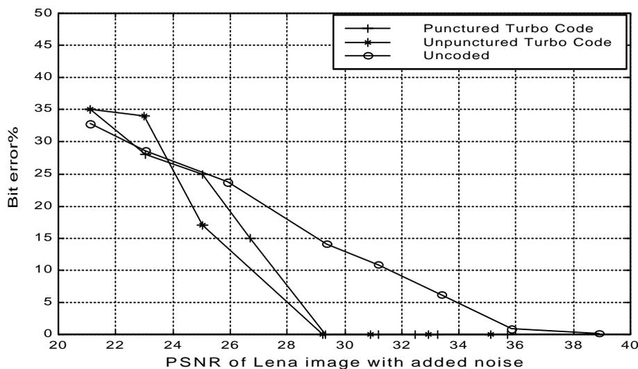
**Figure 4** Bit error rate versus noise addition attack for turbo coded and uncoded messages.
