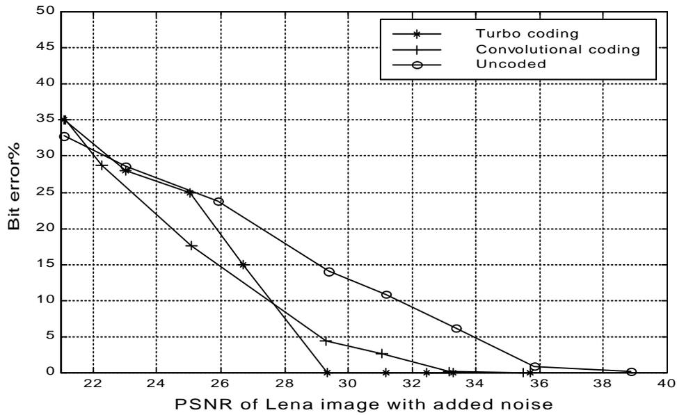
**Figure 6** Bit error rate versus noise addition attack for turbo coded, convolutional code and uncoded messages.
