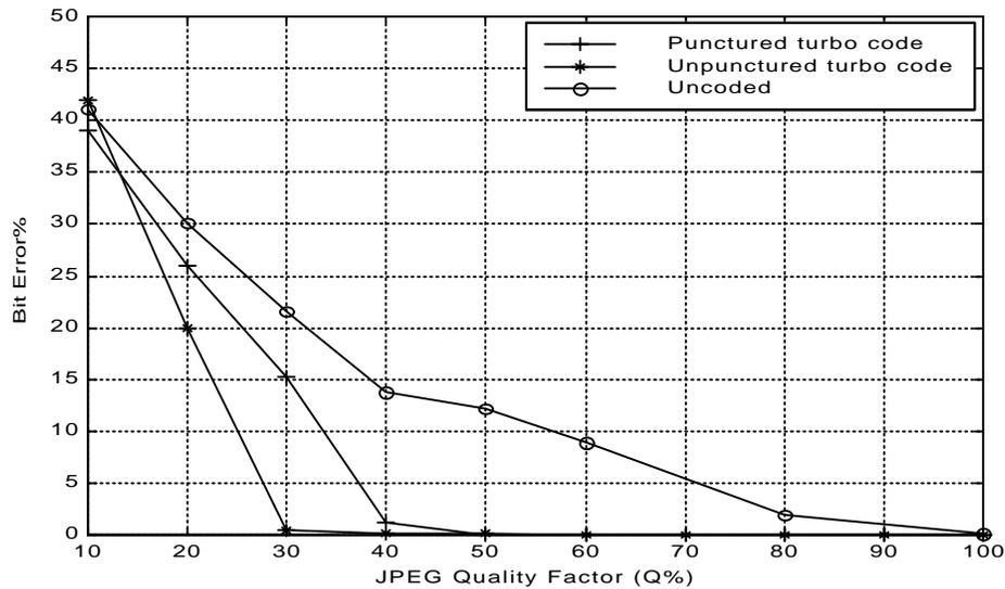
**Figure 3** Bit error rate versus JPEG compression for turbo codes and uncoded messages.
