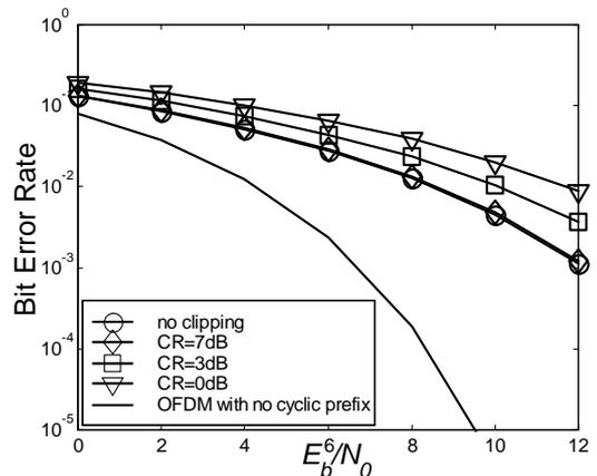
Figure 7: BER versus  $E_b/N_0$  in a two-path channel for varying clipping ratios
