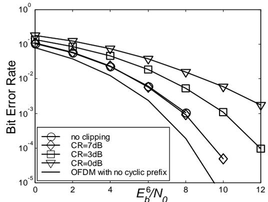
Figure 6: BER versus  $E_b/N_0$  in AWGN for varying clipping ratios
