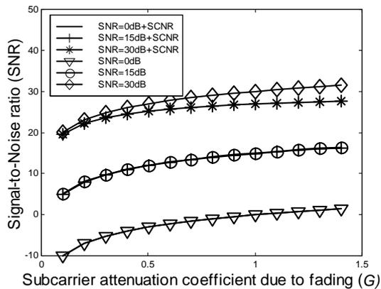
Figure 5: Signal-to-Noise ratio of the received signal in 2-path fading channel
