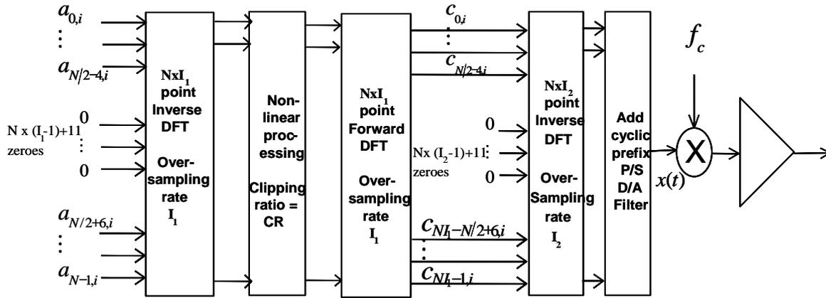
Figure 1. Block diagram of new peak reduction technique
