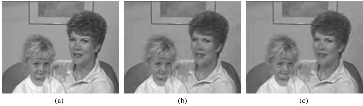
Figure 6: Mother and daughter frame 92, at 30kbit/sec and 10 fps. (a) Original (b) 3-D SPIHT (PSNR=34.62dB) (c) 3-D VSPIHT (PSNR=35.13dB)
