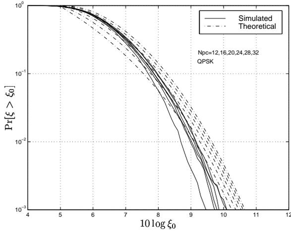
Fig. 2. Theoretical and Simulated CCDF of PC-OFDM.
