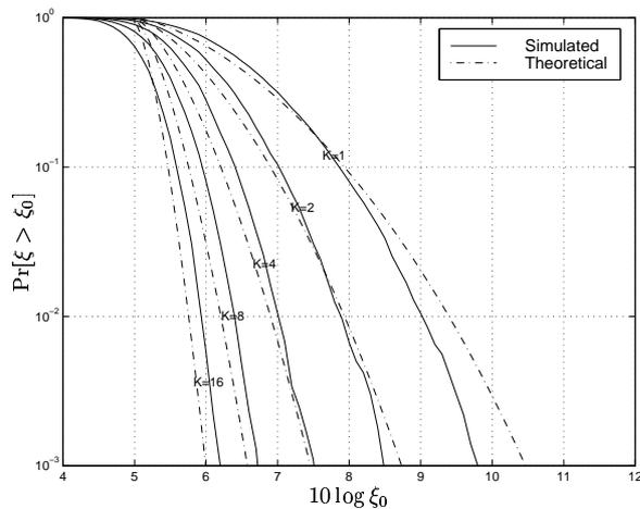
Fig. 5. Theoretical and Simulated CCDF of interleaved PC-OFDM  $N_{pc} = 20$ .
