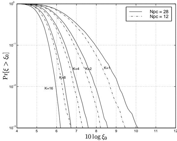
Fig. 3. CCDF of PC-OFDM with interleaving to reduce PAR ( $M=4$ ).
