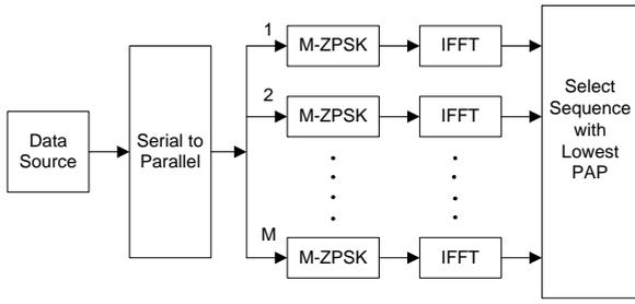
Fig. 1. Block Diagram for Adaptive OFDM Scheme
