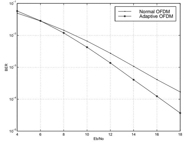
Fig. 6. BER of the Adaptive OFDM Scheme in AWGN channel for  $M = 4$  with  $\varepsilon = 0.1$ .
