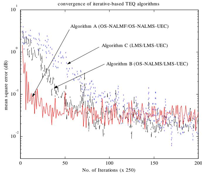
Figure 3. Convergence of iterative-based TEQ initialization algorithms.
