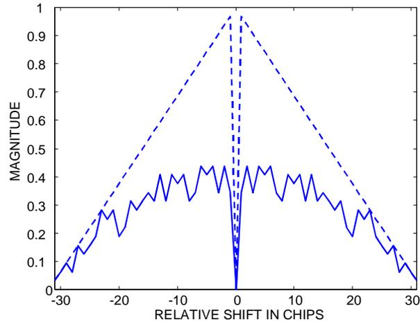
**Figure 1:** Plots of the maximum value of the aperiodic cross-correlation  $ACC_{\max}$  for all possible pairs of the sequences versus the relative shift between them; 32-chip modified Walsh-Hadamard sequences - solid line, 32-chip pure Walsh-Hadamard sequences – dashed line.
