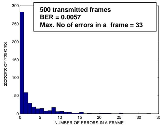
**Figure 2:** Histogram of a number of errors in a transmitted frame for channel 32.
