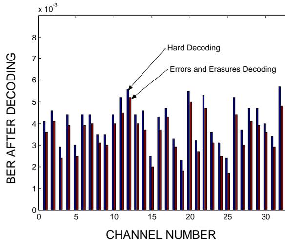
**Figure 4:** Improvement in BER for errors and erasures decoding compared with hard decision decoding for all 32 channels; for all channels the optimal threshold have been applied.
