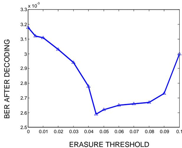
**Figure 3:** BER versus the erasure threshold value for the channel 21.
