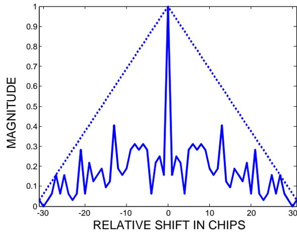
**Figure 2:** Plots of the maximum value of the aperiodic auto-correlation  $AAC_{\max}$  for all possible pairs of the sequences versus the relative shift between them; 32-chip modified Walsh-Hadamard sequences - solid line, 32-chip pure Walsh-Hadamard sequences – dashed line.
