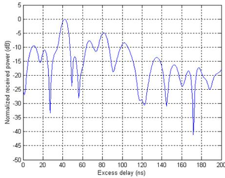
**Figure 7. Power delay profile for transmit position F in the stairwell**
