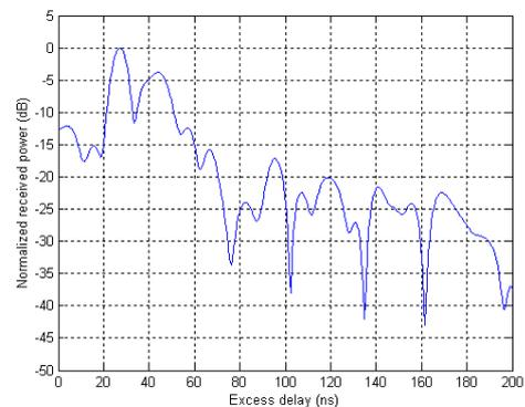
**Figure 5. Power delay profile for transmit position A in the small room**
