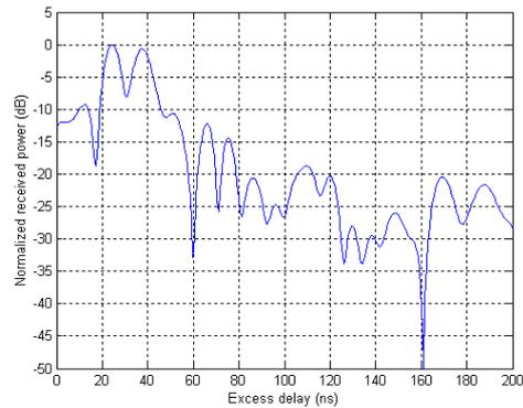
**Figure 9. Power delay profile for transmit position C in the small room**
