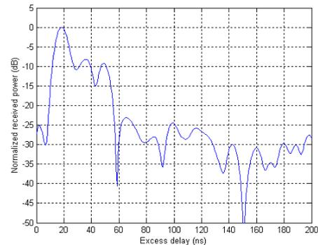
**Figure 10. Power delay profile for transmit position E in the small room**
