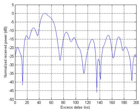
**Figure 6. Power delay profile for transmit position E in the hallway**
